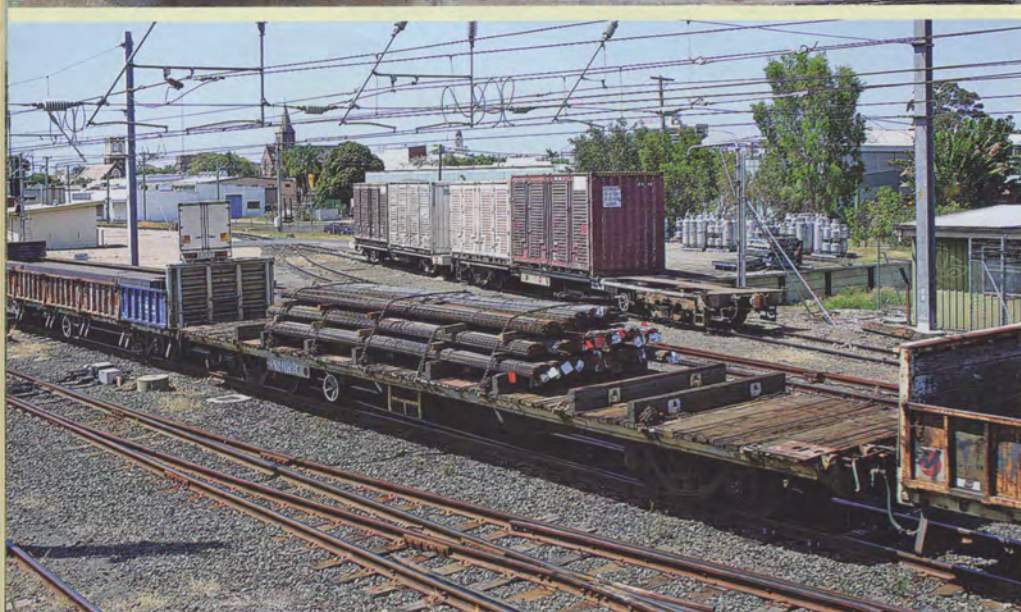
▼ C channel and angle iron loaded in a HWOS open wagon at Acacia Ridge on 11 March 2007. Photo by Arthur Hayes.
