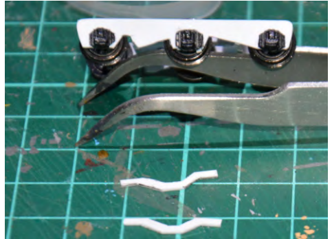
The bogies were mounted off centre to reduce the overhang on curves. The centre wheelset has extra side movement
