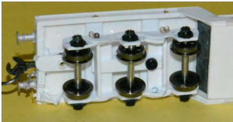
The bogies were mounted off centre to reduce the overhang on curves. The centre wheelset has extra side movement
