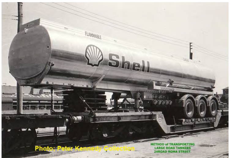
The bogies were mounted off centre to reduce the overhang on curves. The centre wheelset has extra side movement
