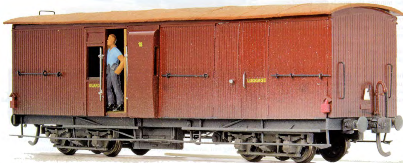
CV 18 was built in 1963 using a surplus carriage underframe (coach CL 18 built in 1886).
