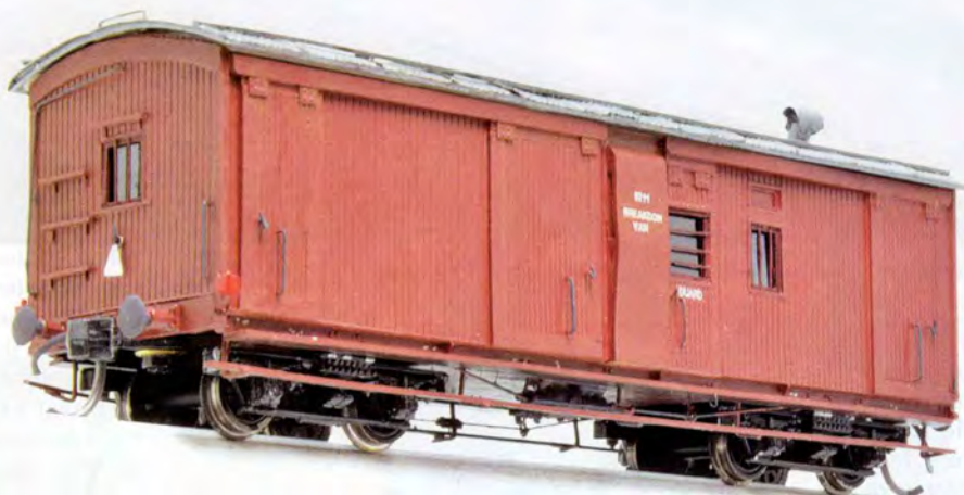
Many small country depots had a stand-alone Breakdown van for quick response to minor, local derailments.
