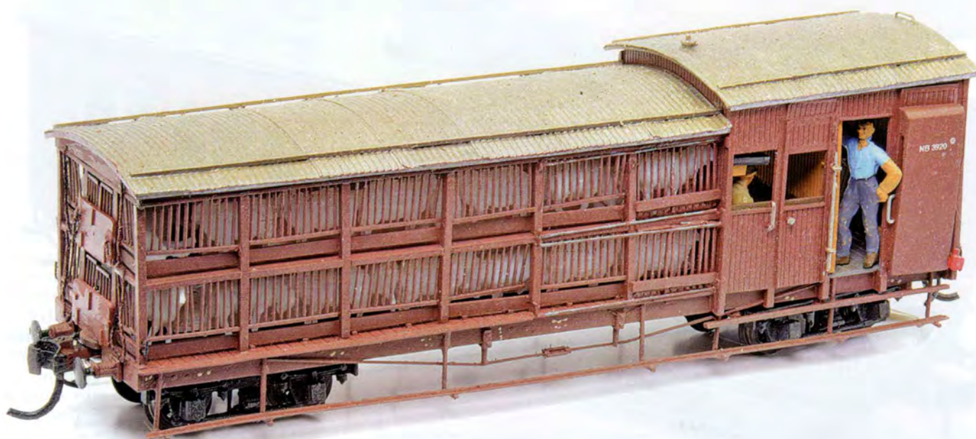
NB No. 3920 sheep van added extra loading (revenue) to a train and provided accommodation for the drover and guard. The vertical bars were made from Ratio 'N' gauge No. 245 Great Western Railway spear fencing kits.
