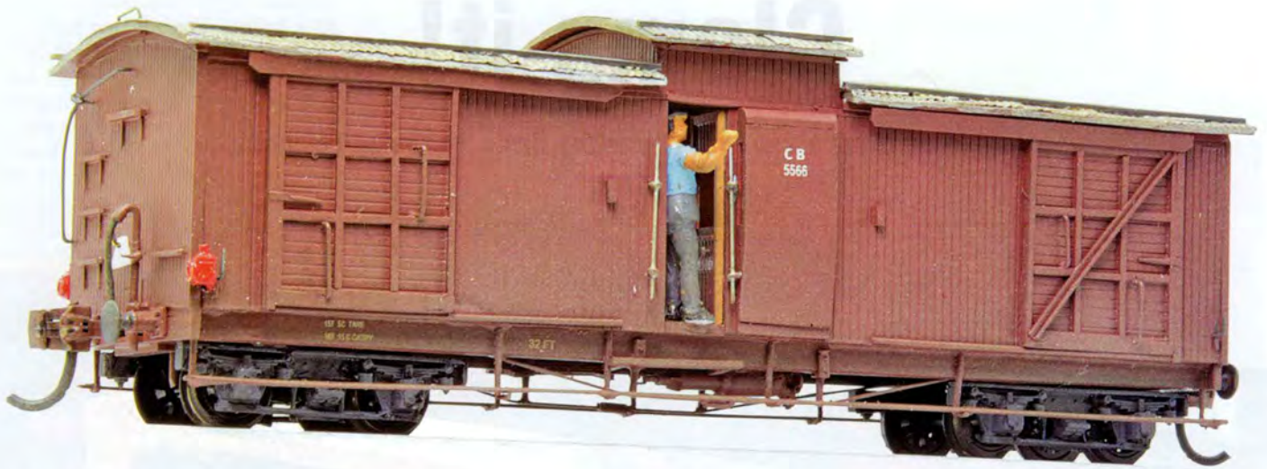
One of many World War two (WW2) conversions, a box wagon converted into a Guards van, CB class. Some of these vans made it to the end of the wooden wagon era as breakdown vans.
