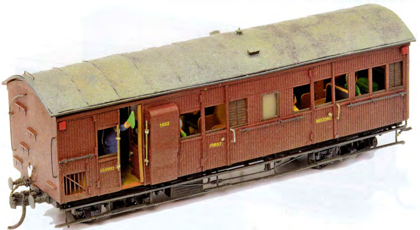
CLV class van (Composite Lavatory Van) No. 1402 for mixed trains with passenger accommodation on branch lines. 20 CLVs were built in 1950/51. In later years, many were modified with the 1st class compartment becoming part of the guard's compartment, making them BLV class vans.
