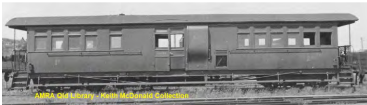
CLV 581 after rebuilt in 1935. Toilets moved to the ends and one dog box. Seven - 1 st and 17 - 2 nd class passengers.
