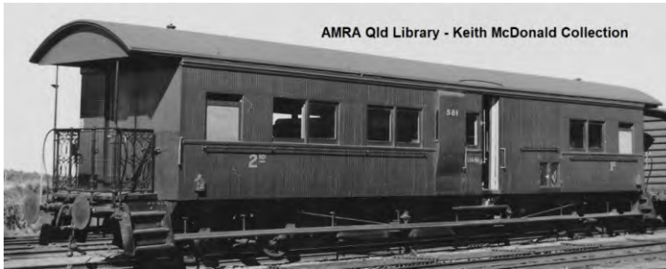
CLV 581 after rebuilt in 1935. Toilets moved to the ends and one dog box. Seven - 1 st and 17 - 2 nd class passengers.
