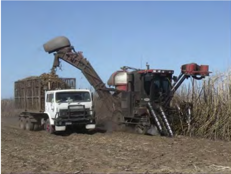
Left: Chopper harvester loading directly into cane bins on truck. The bins are then delivered to the cane railway siding for transport to the mill.
