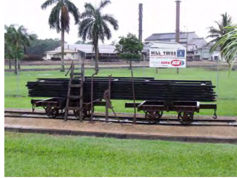
Portable tramway rail was used to get the cane trucks into the canefield for loading
