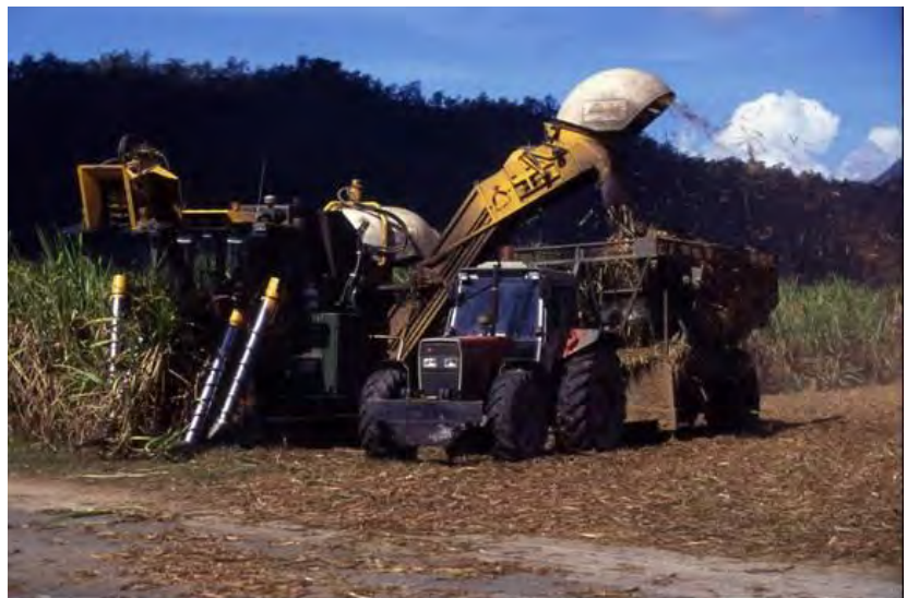
Right: Chopper harvester loading into tractor “haul out” which transfers the cane to cane bins at the cane railway siding.
