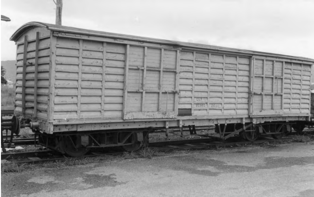
CJFF downgraded and reclassified to CLF (Carrying capacity reduced from 20 t to 8 t).
