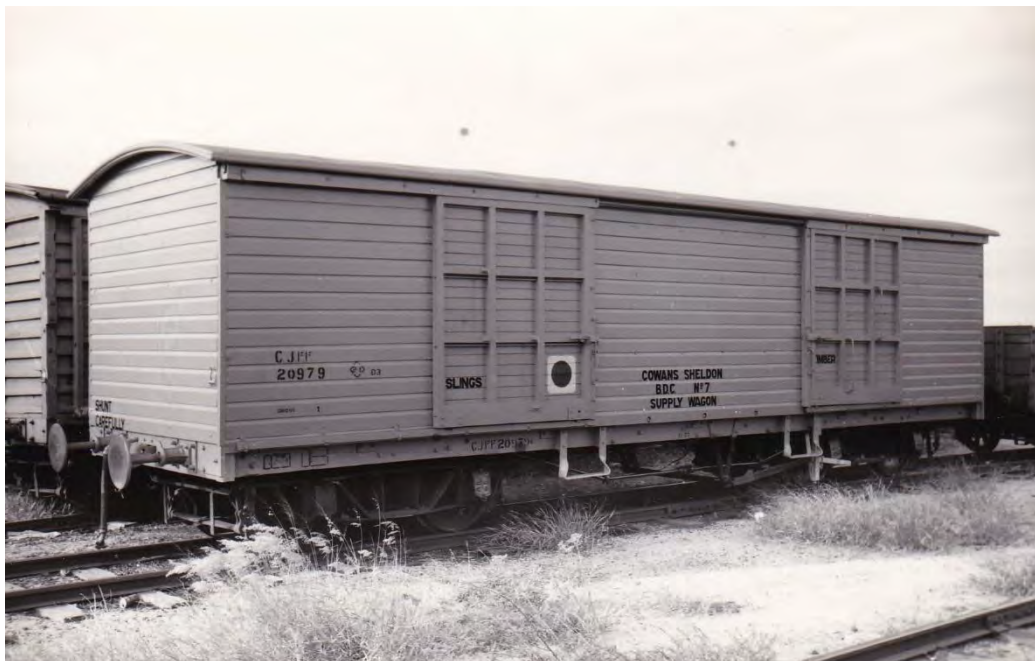
CJFF 20979 with boarded side/ends. Wagon used with ND Breakdown Crane No 7 to carry equipment (Slings/Timber) for derailments. Townsville 79. ( Breakdown Crane were restricted to 60 km/h ).
