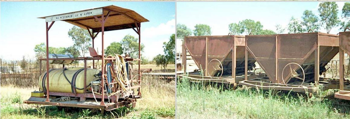
Proserpine Mill, 1997: weed sprayer, ballast hopper, bottom dump mill wagons
