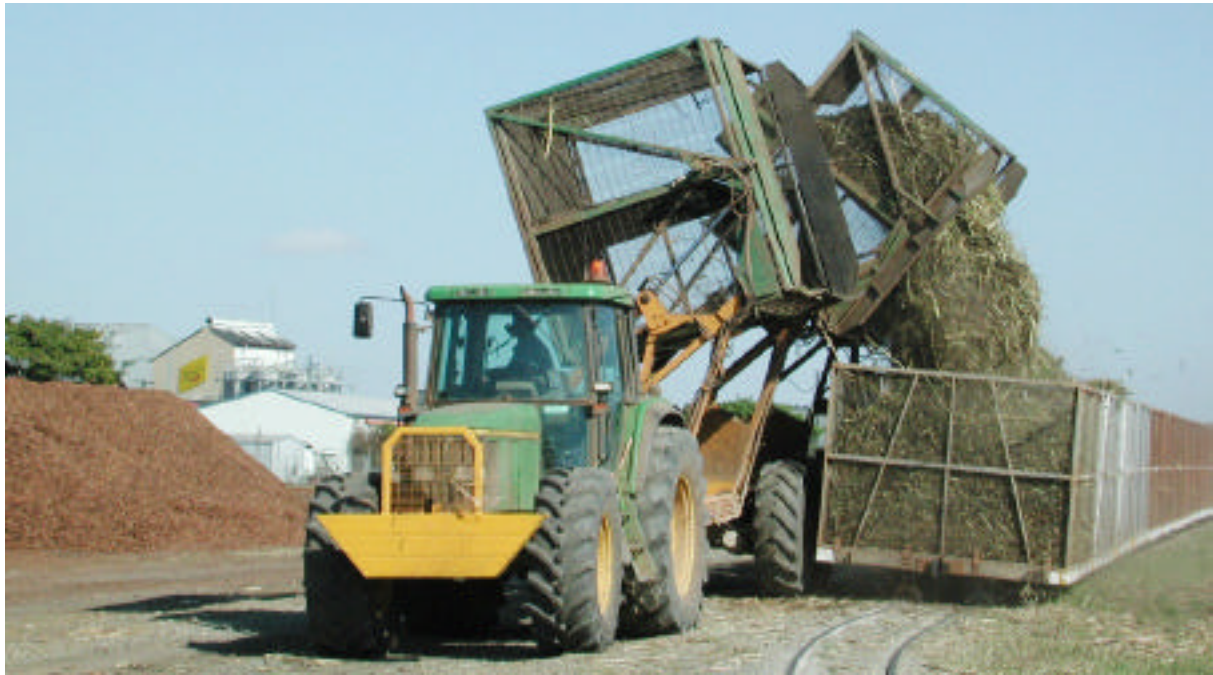
Transferring cane from in-field transporter to cane bins for delivery to mill, 2002
