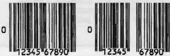
The UPC Symbol decodes into two separate halves, each with a different parity—the central guard bars serving both halves
