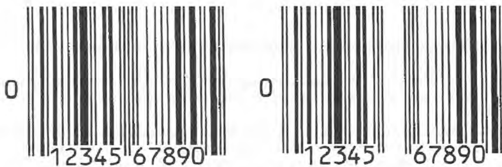
Figure 1: The larger-than-life UPC Symbol on the left, used for identifying grocery items, decodes into two separate halves, each with a different parity. The central guard bars, duplicated in the symbols on the right, serve to delineate both halves.
