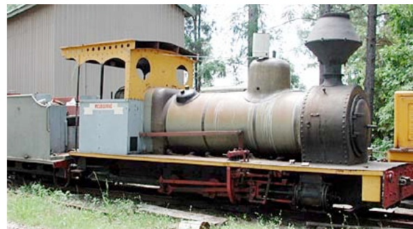
Victoria Mill's 0-6-0 Melbourne , built in 1938 by Hudswell Clarke of Leeds #1701. It's been restored and is one of the two operating steam locomotives on the Australian Narrow Gauge Railway Museum Society's Durundur Railway at Woodford, Qld. Photographer: Lynn Zelmer.
