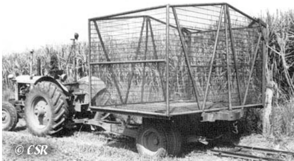
Second generation 3 ton bins utilised Victoria Mill wooden stanchion wholestick trucks. Bins were transported into the fields for filling and then transferred to rail for movement to the mill. CSR photo from the collection of C Hart.
