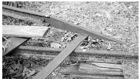
The inclined plane above is one end of a curved section (see also the Orenstein & Koppel illustration on the next page) and slips over a straight section to allow a wagon to be pushed up and over onto the temporary track—usually by man or horse power.
