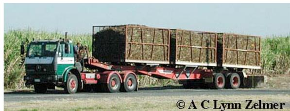
Road transport unit leaving a cane-only ferry and then delivering its bins to a rail transfer point on Fairymead Mill's River Road. Similar units carry cane bins through most mill towns.
