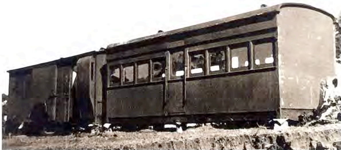
ABOVE: Photographer and date unknown, on stumps at Buderim after the vehicles were out of service. Note differences in the end hardware, door height and name board. The vehicle behind is the brake van. This is the best photo of the First Class Coach in the CaneSIG online collection, Photoshopped from a print in the Ted Ward Collection.
