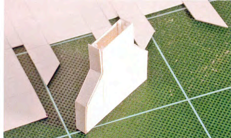
ABOVE: The first chimney was laid out on styrene sheet, cut and assembled with interior square strips reinforcing the corners. Adjacent (joining) angles were adjusted by sanding during assembly, with the near side of the upper portion of the chimney ready for gluing in this view.
