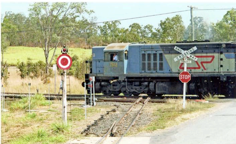
ABOVE: Mackay Sugar, Marian Mill: QR 1512 crossing Marian Mill's 2' line on the North Coast Line near Kuttubal, September 1990. Note the stop signal and cane line check point. Lynn Zelmer photographer.
