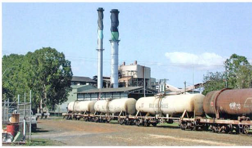
BELOW: Bulk tankers for molasses on Queensland Rail have evolved over the years. This mixed string is outside Proserpine Mill, January 2003. Lynn Zelmer photographer.
