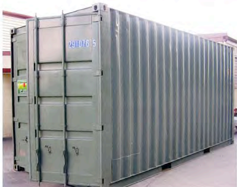
ABOVE: A slightly different door and rib designs appears on this container used by AMIRA(Q) for storage of their exhibition tables and other materials. The roof of this container is not flat; instead it is formed from the same ribbed material as the sides.
