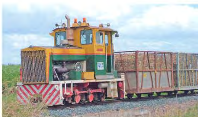
ABOVE: Mackay Sugar 0-6-0 DH No 54 Oakenden (Com-Eng FB3169 of 1963) with the 'One Team' logo, 2005. The white frame and steps helps with night visibility, a particular concern when crossing public roads. Jonathan Bayliss, photographer.
