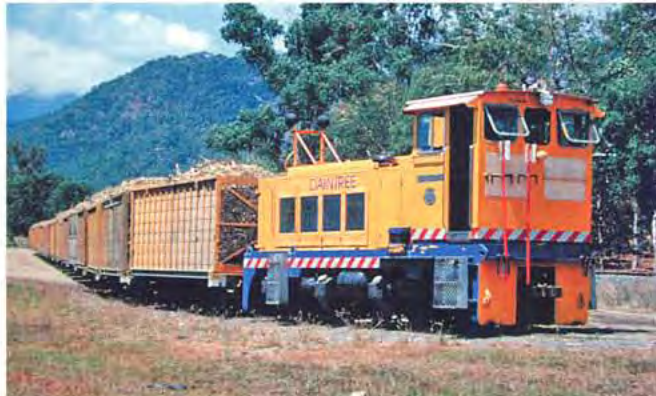
ABOVE: Mossman Mill's 'Daintree' at Mowbray River Road, September 1996. Note that the safety striping appears on both the sides and ends of the loco. The light steps and white panels on the cab back presumably make the loco more visible at night. Greg Stephenson, photographer
