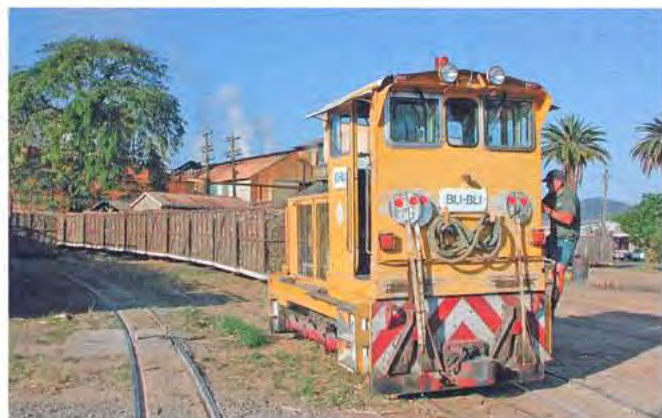
ABOVE: Moreton Mill's livery, Yellow with Black hood top, is perhaps the best known of the sugar mills because of its proximity to Brisbane. Bli-Bli (EM Baldwin, 0-6-0 DH of 1965) gets an early morning start in the mill yard, September 2003, during the last crushing season before the mill's closure. Contrary to general industry practice, the loco has its name on the rear of the cab as well as the sides. Bli-Bli, also known as Bli Bli, was on loan to Millaquin Mill for a short period in 1999 and following Moreton Mill's closure was sent to Bingera Mill. Lynn Zelmer, photographer.
