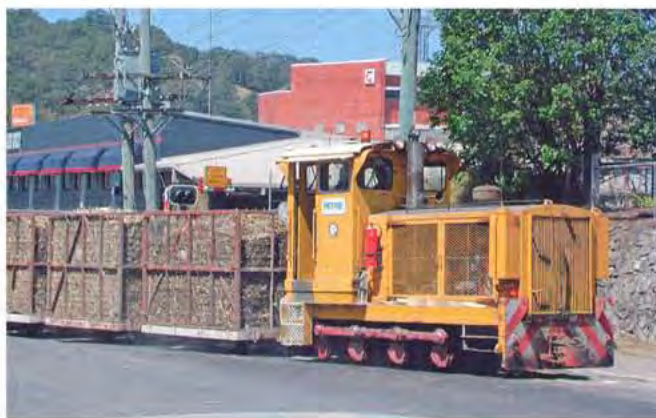
ABOVE: Petrie, the locomotive: Moreton Mill's Petrie (EM Baldwin 0-6-0 DH of 1968) approaching the mill in September 2003, just months before the mill was closed. The loco was built on the frame of a 915mm gauge loco used by a Snowy Mountains Scheme contractor but is quite similar to Bli Bli. It appears to have a light grey cab roof and visors, with a darker grey on the top of the bonnet to reduce glare for the driver. Lynn Zelmer, photographer.
