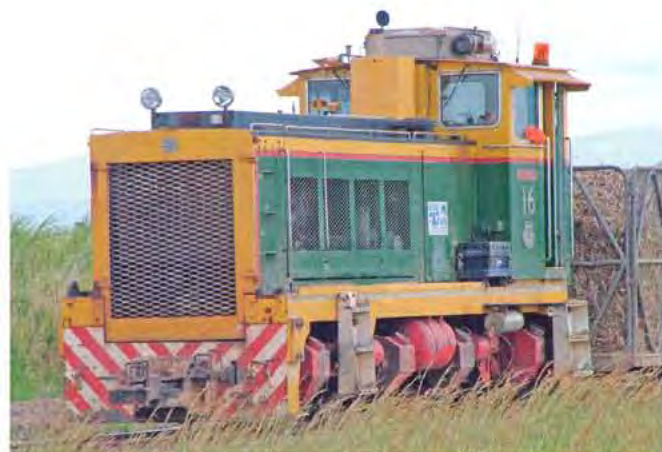
ABOVE: Mackay Sugar B-B DH loco No 16 Charlton (EMB 9562.1 6.81 of 1981), with an alternate location for the 'One Team' logo, 2005. The loco frame also appears to have a reflective stripe down its length for better night visibility, Jonathan Bayliss, photographer.
