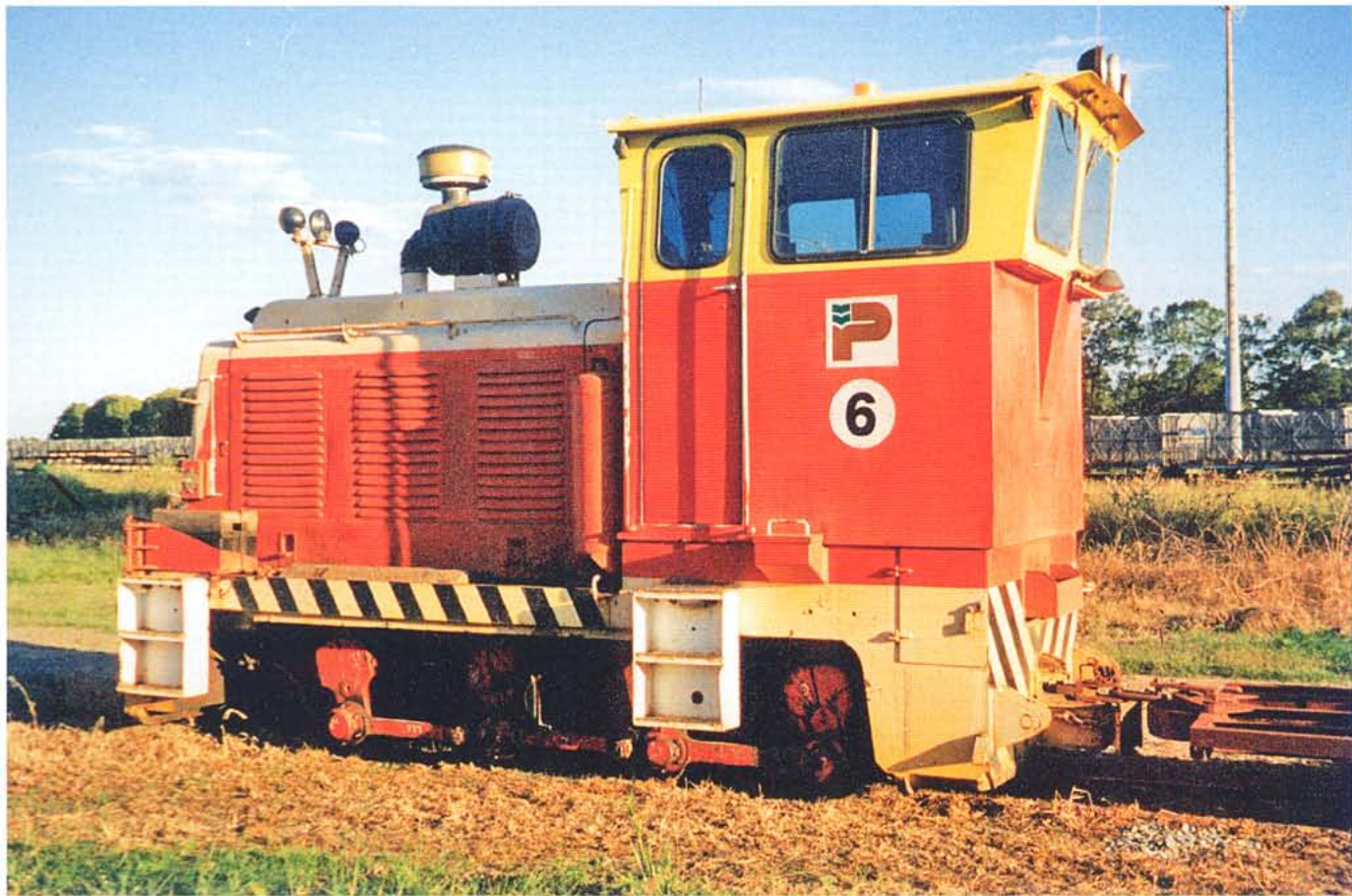
ABOVE: Proserpine Mill No 6 stabled near the Navy Shed, March 2002. While it may simply be a faded yellow, the top of the hood appears to be a matte cream colour. The skirting around the frame and the side safety striping provides another variation while the rear stripes appear to be white. Note the triple lights, high enough to shine over the bins, the 'V' safety striping on the rear and the striping on the frame. David Rowe, photographer.
