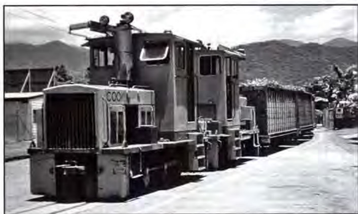
ABOVE: Mossman Mill, Mossman, 1995. Cook (0-6-0DH, Com-Eng, 1964) and Ivy (0-6-0DH, Com-Eng, 1965), fitted for multiple unit operation in the 1980s, with a rake of canetainers. Greg Stephenson photographer.
