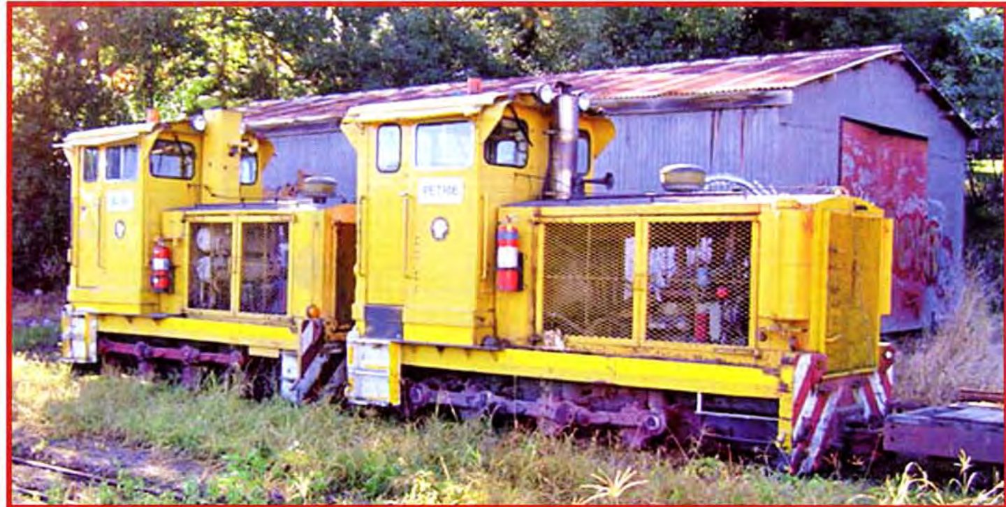
ABOVE: Moreton Mill: Petrie (right, EM Baldwin 0-6-0 DH of 1968) and Bli-Bli (EM Baldwin 0-6-0 DH of 1965) at the Howard St yard, 8 June 2004. Many of these locomotives ran with their bonnets doors open or fully removed; by 2004 Workplace Health and safety had required such openings to be screened. Carl Millington photographer.
