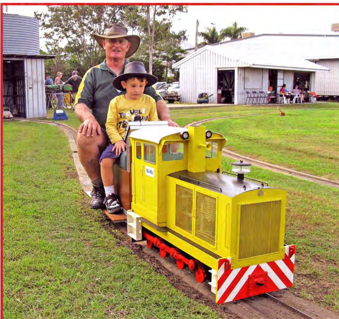
LEFT: Edward Millington with a young railfan and his 5" gauge model of Moreton Mill's Bli-Bli (EM Baldwin 0-6-0 DH of 1965), seen operating in Rockhampton, June 2008. The ride-on trailer includes a full control panel and the loco will soon be fitted with yellow flashing safety lights as per the prototype. Lynn Zelman photographer.
