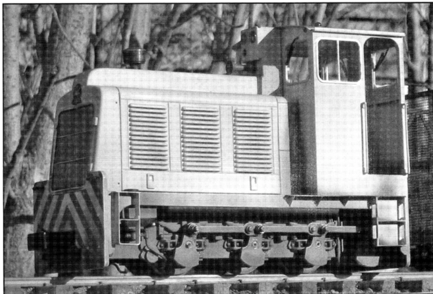
BELOW: Limited run 0-6-0 Clyde DH locomotive in SM32 from Tim Boulton's Tootle ( www.tootleng.com ). Scaled at 16mm = 1" (1:19 scale) and using 32mm track this provides a true to scale 2' gauge.
