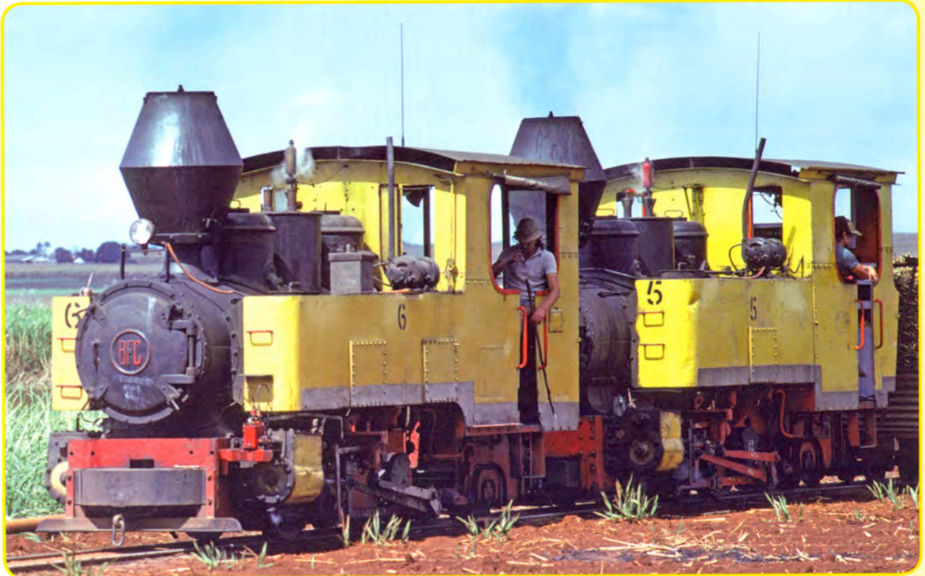
Nipper (BFC 3 of 1952, 0-4-2T) and Dobbin (BFC 6 of 1952, 0-6-2T) double head into Qunaba Mill with a full rake of cane bins, 1977. Ross Driver photo
