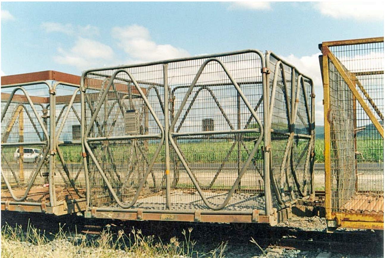
Marian Mill 4 ton bin; note extended sides on bin at left to increase capacity
