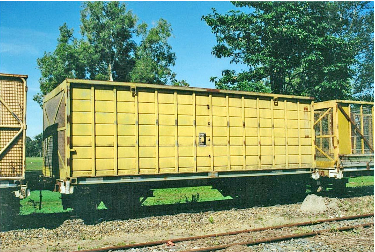
Mossman Mill nine tonne canetainer
