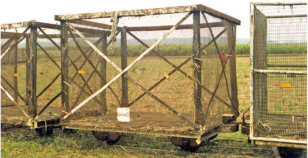
Early Mourilyan Mill cane 2.5 ton bin built on ex-wholestick truck frame
