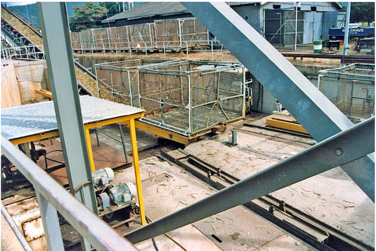
Cane bin traverser on the dead end mill layout at Mulgrave Mill
