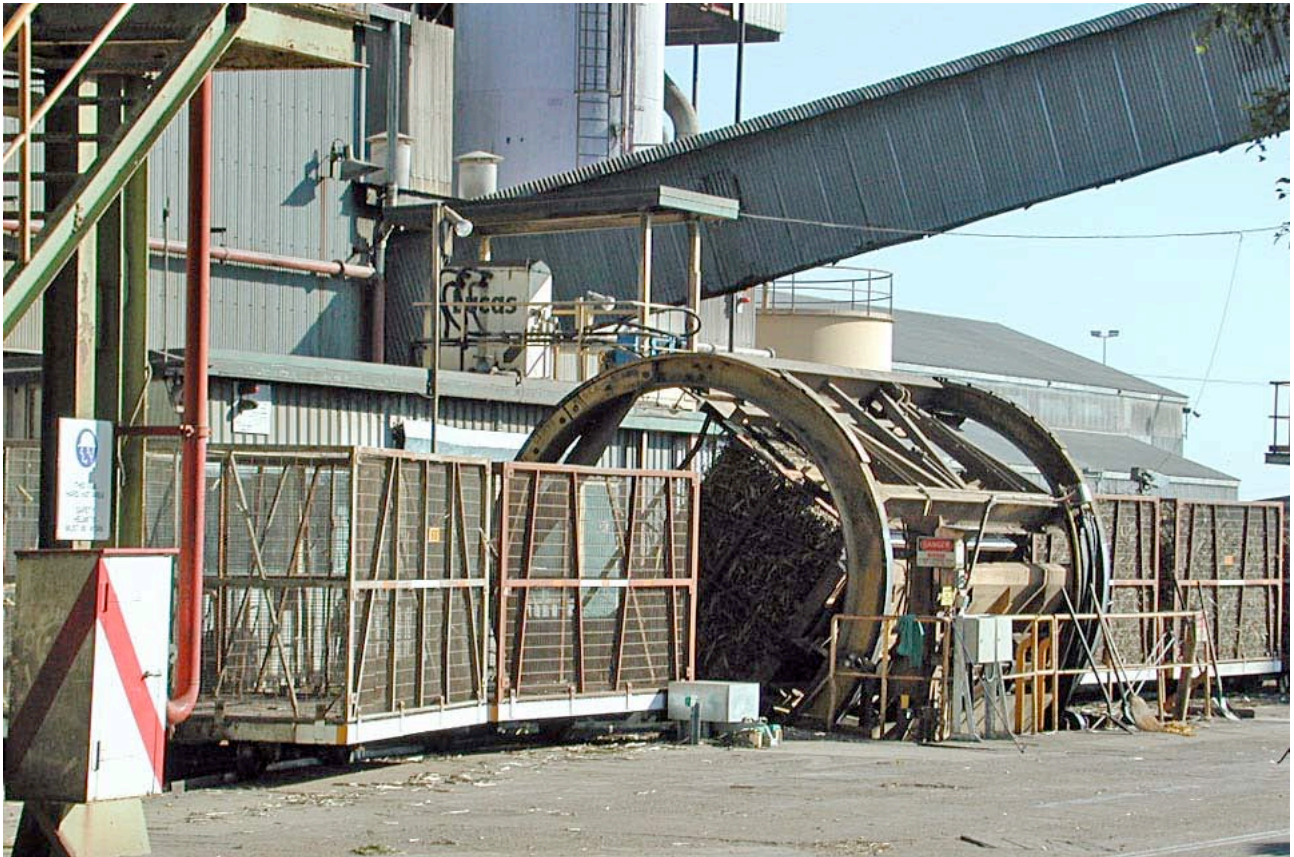
Bin being tipped at Fairymead Mill, July 2002. Lynn Zelmer, photographerr
