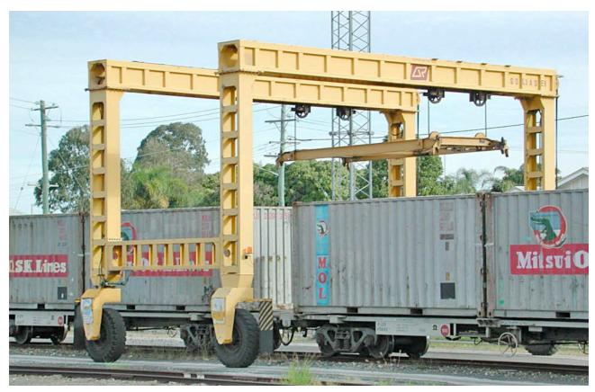
ISO standard container handling crane (above and bottom previous page) for transferring containers to/from rail/road transport, Bundaberg 2003. Lynn Zelmer photo.
