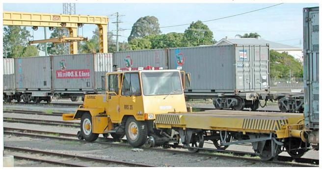
Linmac rail tractor with LSR (loco shunt runner) wagon used as a buffer when shunting, Bundaberg 2003. Lynn Zelmer photo.
