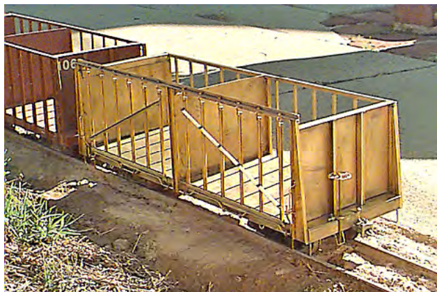
Unpainted 1:20.3 two compartment bogie cane wagon built in brass by Jim Petropulos of Los Angeles. See Handbook 19 for details.
