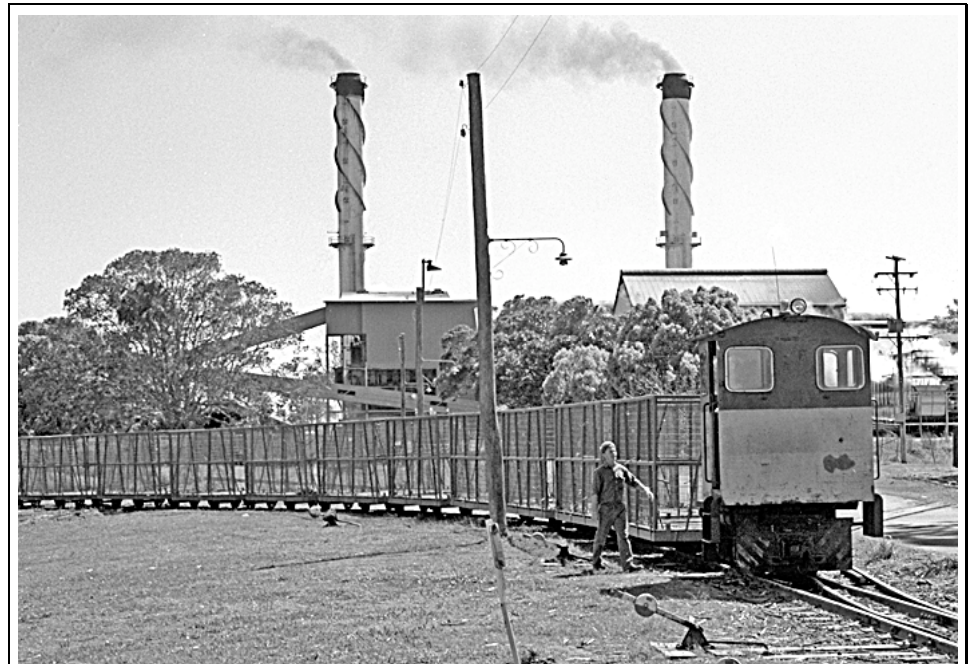
Tiny ComEng-built 4wDM locomotive shunting a rake of empty cane bins at the mill.
