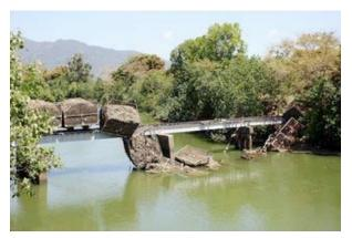
**Off the rails:** Cane bins dangle into the water from the Thomatis Creek cane line bridge and others lie submerged after a wheel came off a bin
