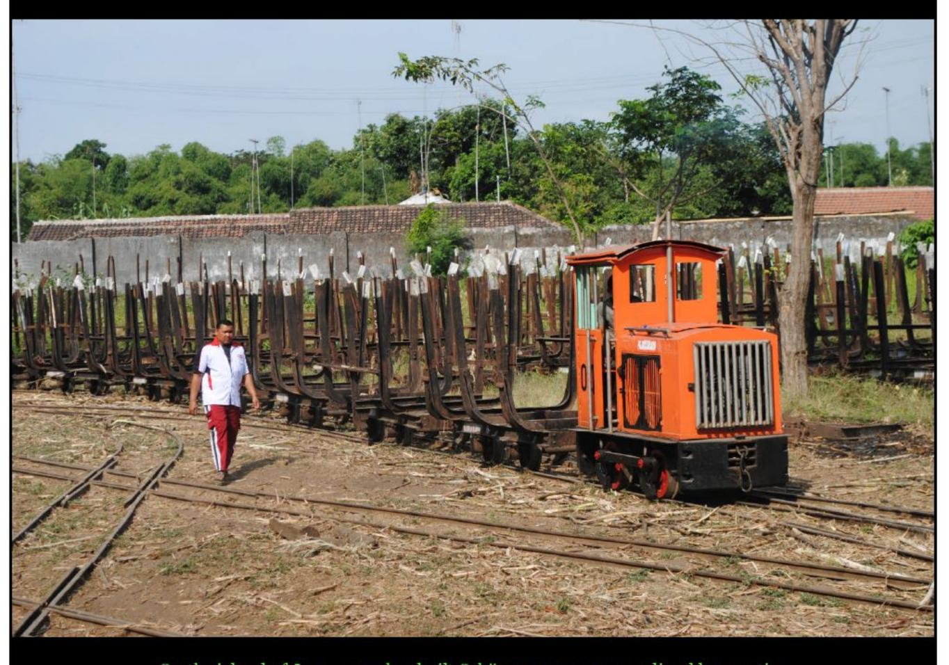
On the island of Java, a much rebuilt Schöma 700mm gauge diesel locomotive shunts empty cane trucks at Padjarakan sugar mill on 20 July 2012.
