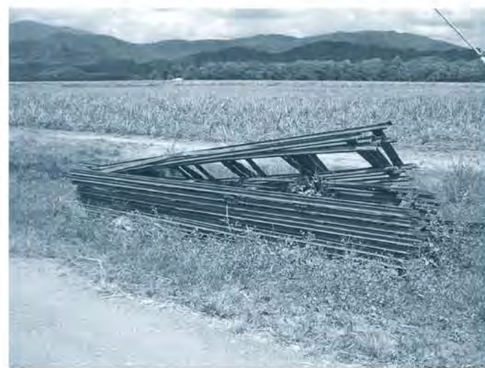
ABOVE: Close-up of portable rail sections with shallow inverted "W" shaped sleepers, PG Karangsuwung, Java, 2008. The bolt and square washer perform the same function as a spike or track clip. There appears to be some variation in sleeper spacing as well as bent sleepers and wear on rail ends. John Browning photographer.
