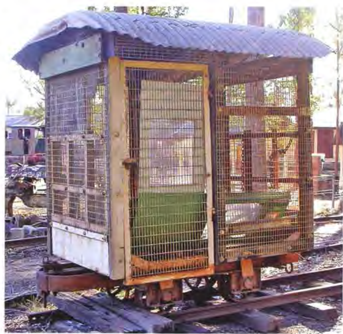
ABOVE: Ex-Moreton Mill 4 wheel gas wagon, now filled with junk, at Durundur Railway, Woodford (Australian Narrow Gauge Railway Society), July 2007. While this wagon is built on an old wholeshtick truck with metal uprights, a reasonable model could be built to fit almost any 4 wheel from a Rugga-type chassis to a cane bin underframe.
