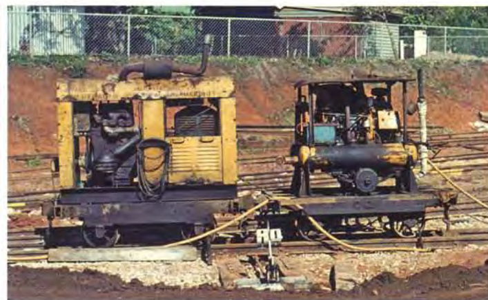
BELOW: Moreton Mill: both generator and compressor are mounted on small 4 wheel chassis and could easily be modelled with either a Rugga-type or ex-wholestick truck. Greg Stephenson photographer, 1982.
