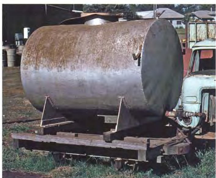
ABOVE: This Bingera Mill water tank is mounted on what appears to be a timber wholestick truck. Probably the most challenging part of modelling this wagon would be the pipe fittings and hose as suitable tanks could come from a variety of HO scale sources or be easily scratchbuilt, Greg Stephenson photographer.
