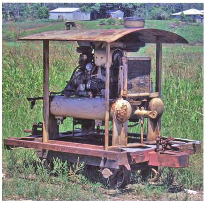
ABOVE: This Bingera Mill water tank is mounted on what appears to be a timber wholestick truck. Probably the most challenging part of modelling this wagon would be the pipe fittings and hose as suitable tanks could come from a variety of HO scale sources or be easily scratchbuilt, Greg Stephenson photographer.
