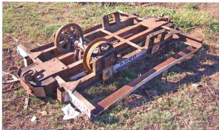
ABOVE: The underside of a FSC steel wholestick truck showing the centre beam and how the wheelsets are mounted, Lautoka Mill, September 2007. The top side of a similar truck appeared in NGDU 24. Lynn Zelmer photographer.
