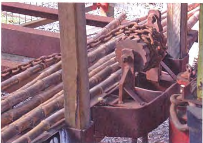
BELOW: Close-up of ratchet system for Moreton Mill steel wholestick truck at Nambour Museum, 2006. The chain was thrown over the load of cane, attached to a hook at the far end, and then tightened to hold down the load. Lynn Zelmer photographer.
