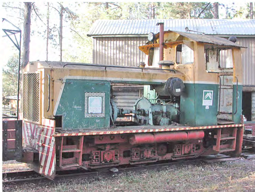
ABOVE: Bundaberg Foundry 6w DM Jenbach D2 ex-Eton, Cattle Creek and Marian Mills. Now named Netherdale and sporting a ComEng bonnet and cab, the loco is preserved at the Durundur Railway (ANGRMS), Woodford Qld. Lynn Zelmer, photographer.
