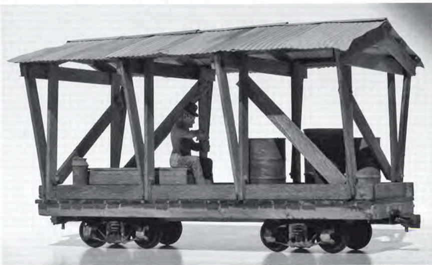
BELOW: Fiji-style On30 personnel car, built on a Mountain Blue Miniatures underframe kit. The navy is sitting on a 32" x 5' x 17" high wooden box, also used for storing tools. Details include Grandt Line nut, bolt and washer castings; barrels; fire extinguisher; petrol cans; and a 'begging' setter dog. I still have to apply dry weathering colours to tone down the colours and age the woodwork. Eventually scaling almost 13' over the eaves, the car is too wide to operate on my layout, but looks good on a display diorama. Lynn Zelmer, model builder and photographer.
