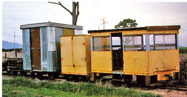
ABOVE: Navy wagons at Marian Mill; 13 Aug 1986. The wagons on the left are for carrying tools and other materials to a work site. The crew car on the right, whether self-propelled or loco hauled, provides transport to the work site, shelter from the elements and serves as a lunchroom. Greg Stephenson, photographer.
