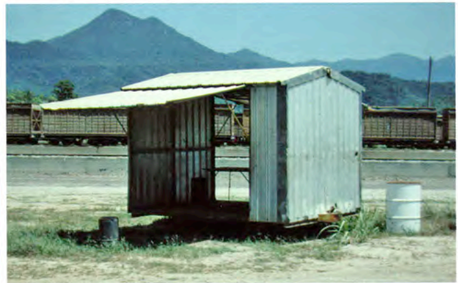
BELOW: A basic crew car, perhaps using a commercial garden shed, on an ex-cane bin underframe or the equivalent. Mossman Mill, Mowbray area (8 Oct 1994). Greg Stephenson, photographer.
