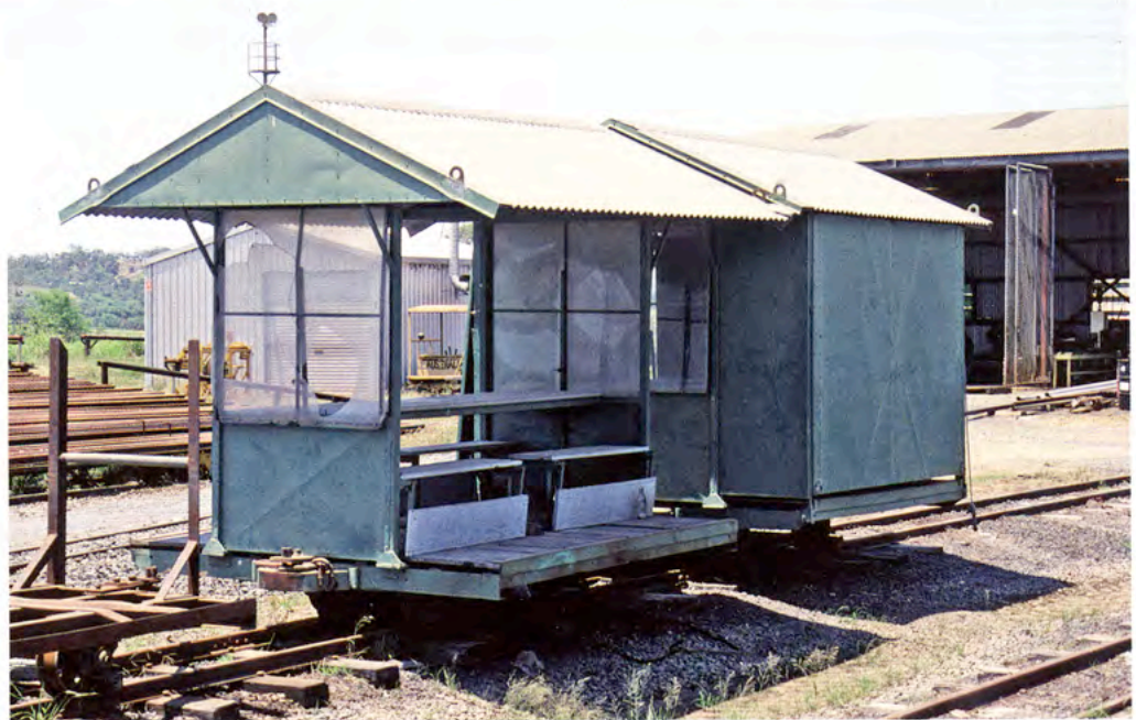
RIGHT: Two Farleigh Mill navy wagons obviously built on ex-cane bin underframes (18 Oct 1997). Both appear to be constructed of square steel tubing with pressed steel sheeting and a narrow corrugation metal roof. The far wagon likely has a single door on the other side and would be used for hauling tools and work materials. The nearer 'toast rack' crew car has tool boxes under the seats as well as a centre table. For a model the most difficult tasks would likely be simulating the pressed steel ridges and spot welding marks. Greg Stephenson, photographer.
