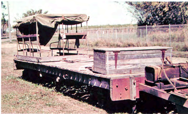
ABOVE: Today's health and safety regulations wouldn't allow you to ride on this Fairymead Mill navy wagon, photographed in 1981. It transported navy tools and materials, and provided shelter from the elements. For modelling purposes the length of the flat car is not important, although it should be remembered that most mill and shire equipment was relatively short. Greg Stephenson, photographer.
