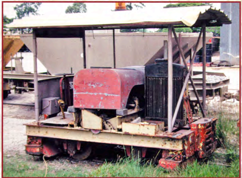
ABOVE: Simplex 'Smokey' (Motor Rail Ltd 4wDH 4054 of 1926, originally petrol) with its distinctive longitudinal radiator at Victoria Mill, 26 October 1996. Note the end buffer with its choice of coupling heights. In the 2000 locomotive list, Victoria Mill still had two operational Simplex 4wDH locomotives and a third had been converted to an unpowered ballast plough. By 2001 'Smokey' had been sold to a mill worker and dismantled to salvage the Dorman diesel engine. Greg Stephenson, photographer.
