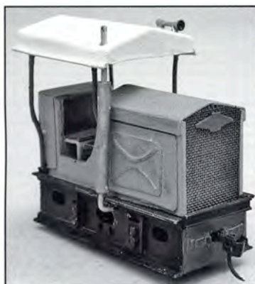
LEFT: Malcolm Moore 4wDM in 7mm scale (On16.5, 1:43), built by John Armstrong using a resin chassis, a vacuum formed plastic roof, and a Bachmann HO 44 ton bogie mechanism. Lynn Zelmer, photographer.
