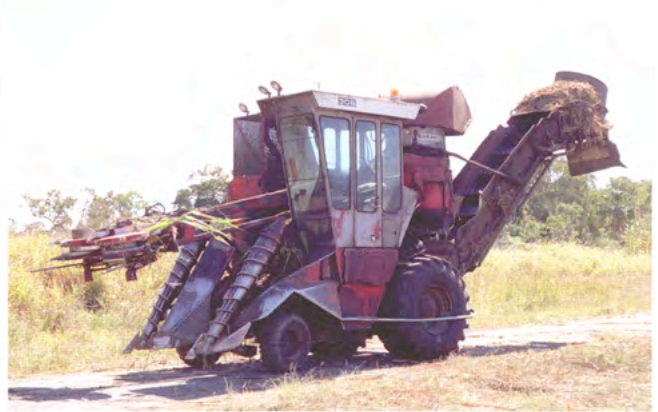
ABOVE: Massey-Harris Model 305 wheeled cane harvester, front view with the topping mechanism raised part way to cutting height, c 1990.
