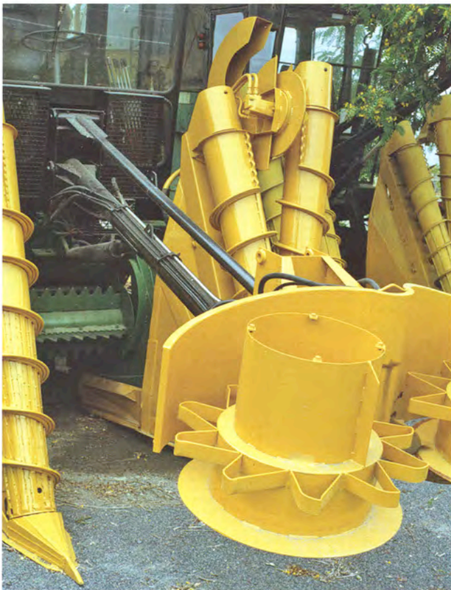
ABOVE LEFT: Austoft 7000 mechanism for topping the cane during harvesting. The topping mechanism is raised to an appropriate height to optimise the amount of harvestable cane while removing the top leaves.
