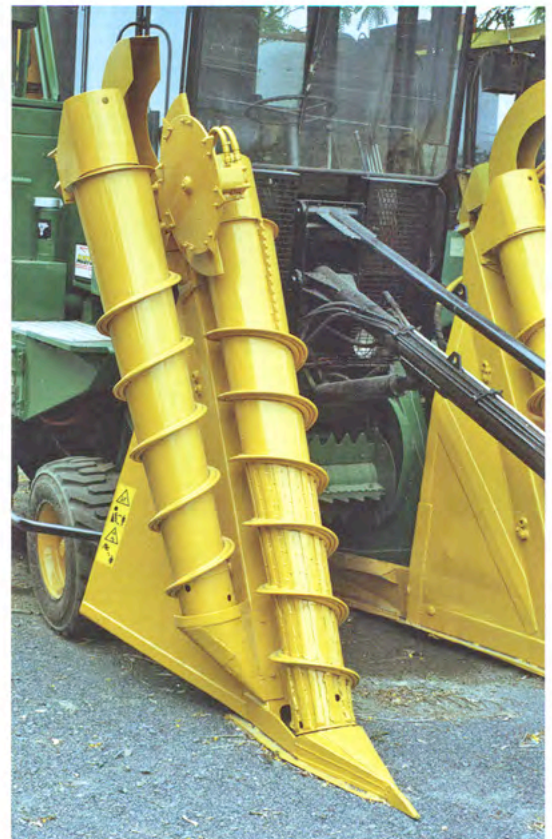
ABOVE LEFT: Austoft 7000 mechanism for topping the cane during harvesting. The topping mechanism is raised to an appropriate height to optimise the amount of harvestable cane while removing the top leaves.
