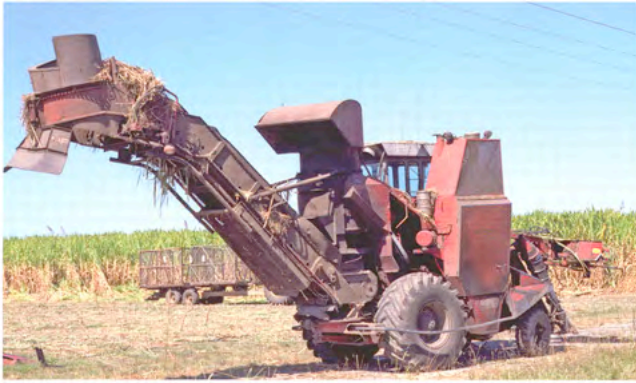
ABOVE: Massey-Harris Model 305 wheeled cane harvester, back view, c 1990. The chopped cane is discharged out the bottom of the elevator mechanism, which can be rotated over the accompanying bin. Trash is blown out of the hood located above and behind the cab.
