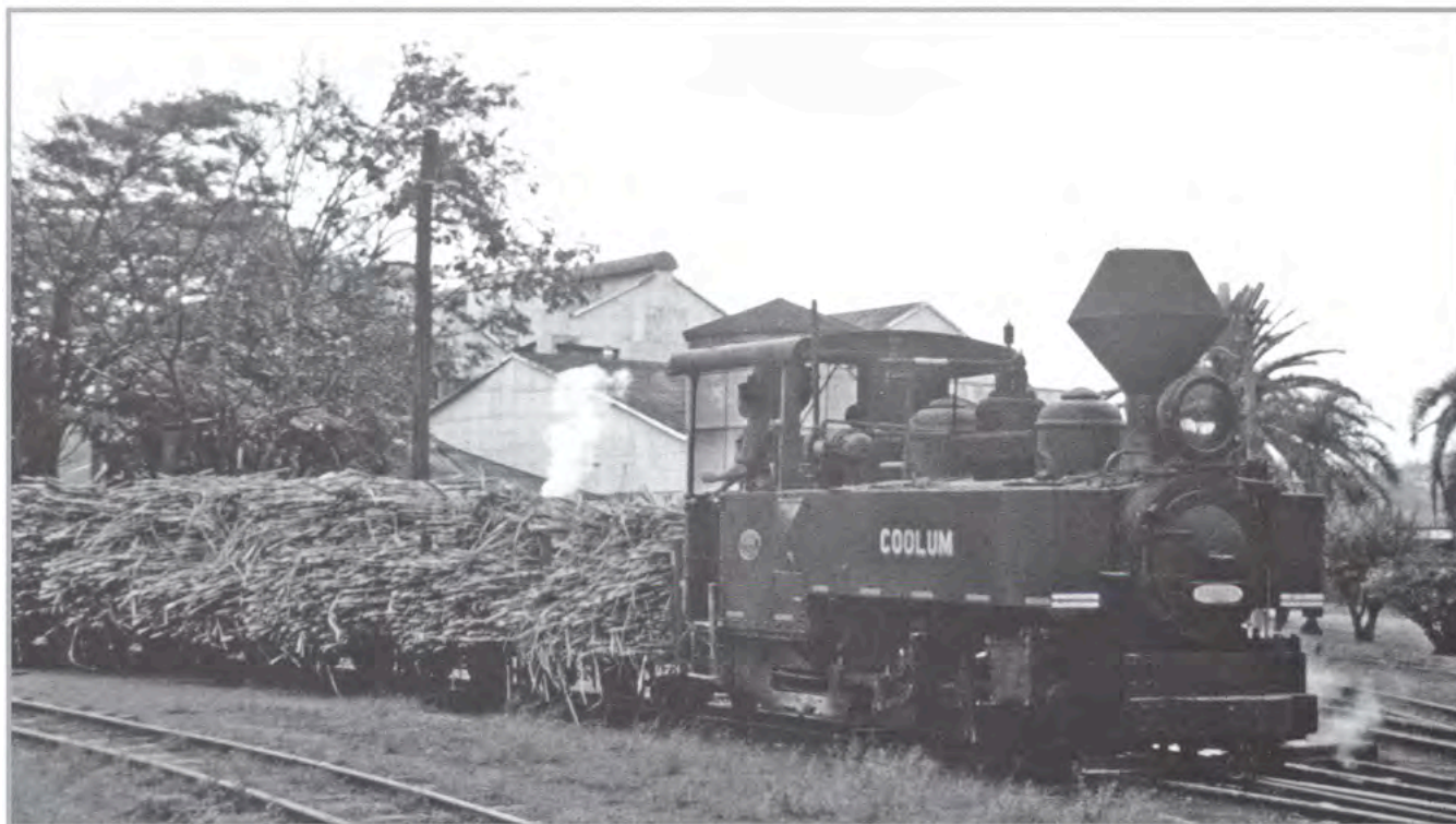
ABOVE: Moreton Mill's Coolum (Fowler 0-6-0T) with a rake of wholestick trucks at the mill, undated. Photo No 3002 A Sydney, G Hughes Production from the John Browning Collection.
