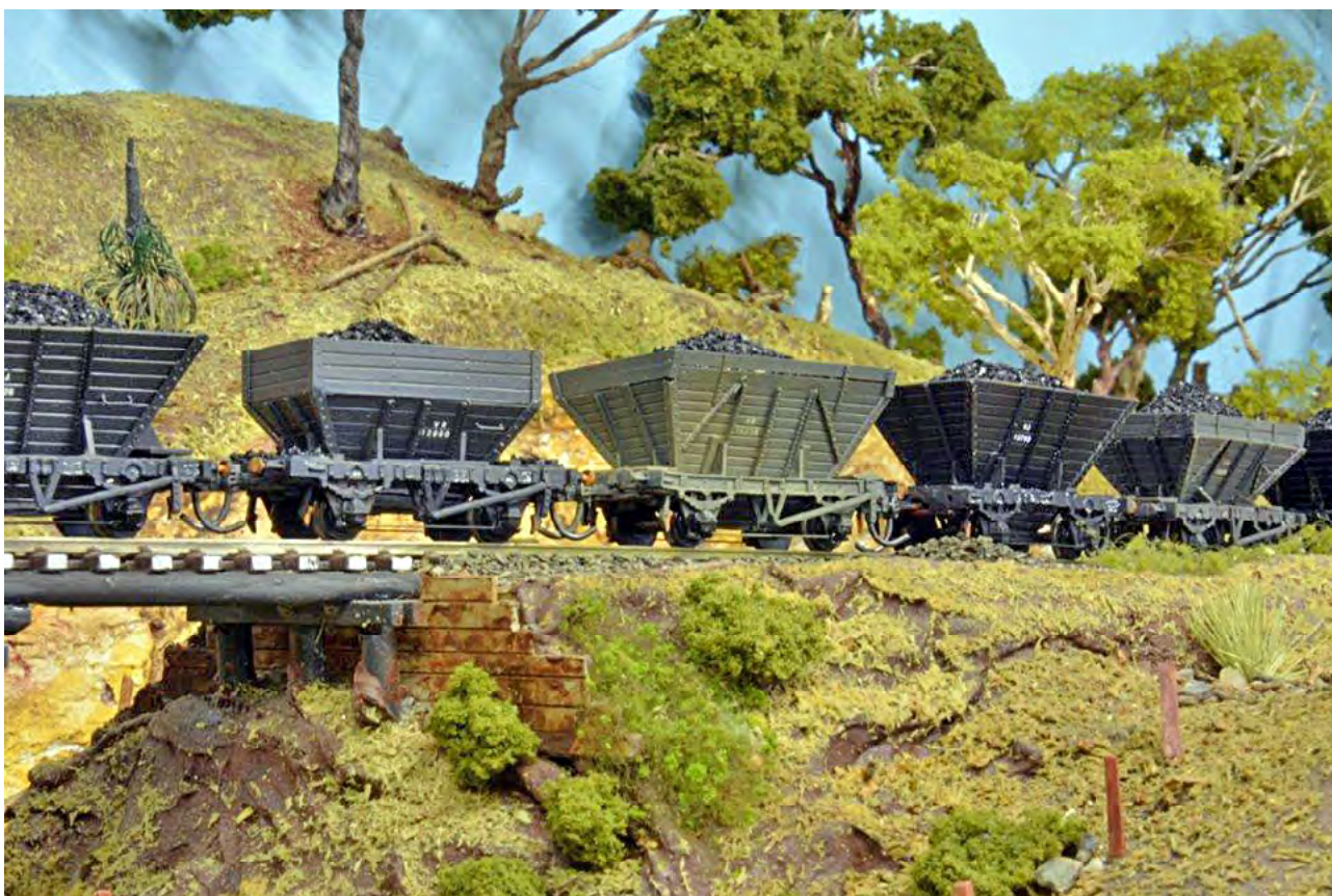
The VJM bodies (above) were scratch built from styrene sheet vacuum formed over a wooden block and detailed. The wooden hoppers (below) were scratch built with scribed siding. All are weighted to 23-25 grams.
