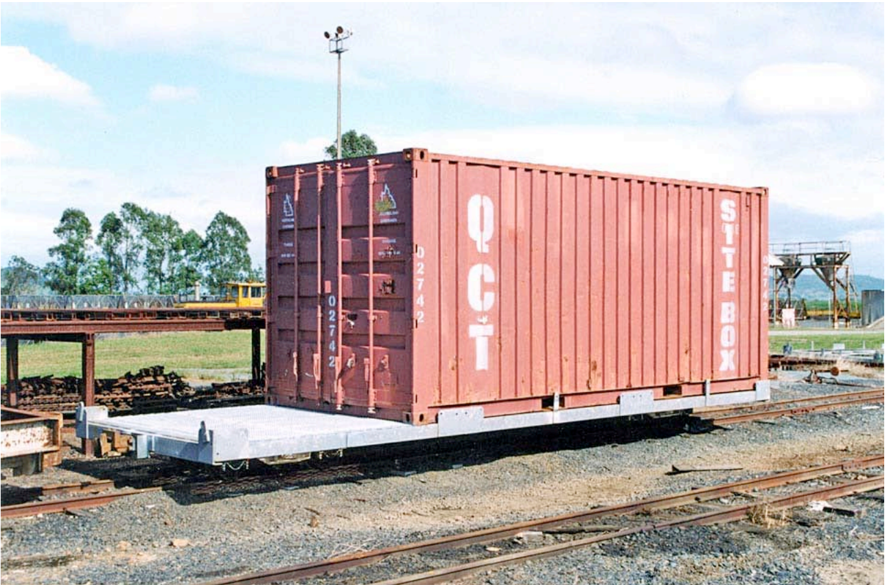
14 ton bogie cane bin frame fitted with a 20 foot container, Farleigh Mill
