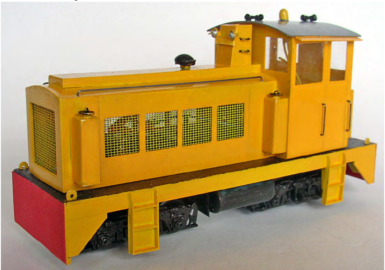
Jay's almost completed 7mm Coolum model. Note how square and even the window and bonnet holes are, the result of careful planning and Jay's use of scrapbooking punches.
