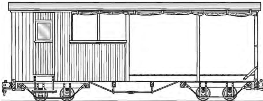
Mapleton Tramway 24' 2" long, 7' wide (over guard's enclosures) passenger and guards van, likely with longitudinal seating. Jim Fainges drawing from K McDonald dimensions.
